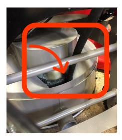
7. By following the dimensions provided in the image below, drill a (3/8") mounting hole for the water flow adjustment cable. When you've fastened the flow control cable, be sure to keep it as free as possible, allowing the cable to smoothly be pulled and pushed inside the cable housing.
